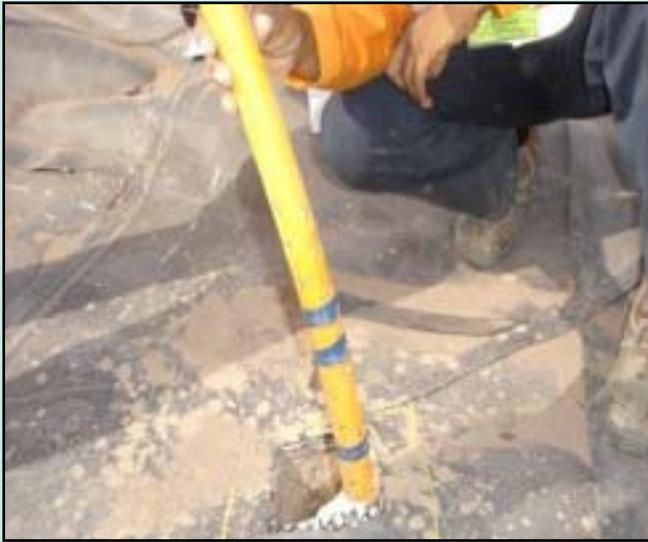
Figure 4 - Moisture sensor installation , April 2007
